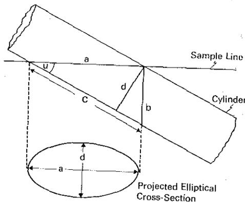
FIGURE 1. The elliptical cross section at the intersection of sample line and cylinder.
