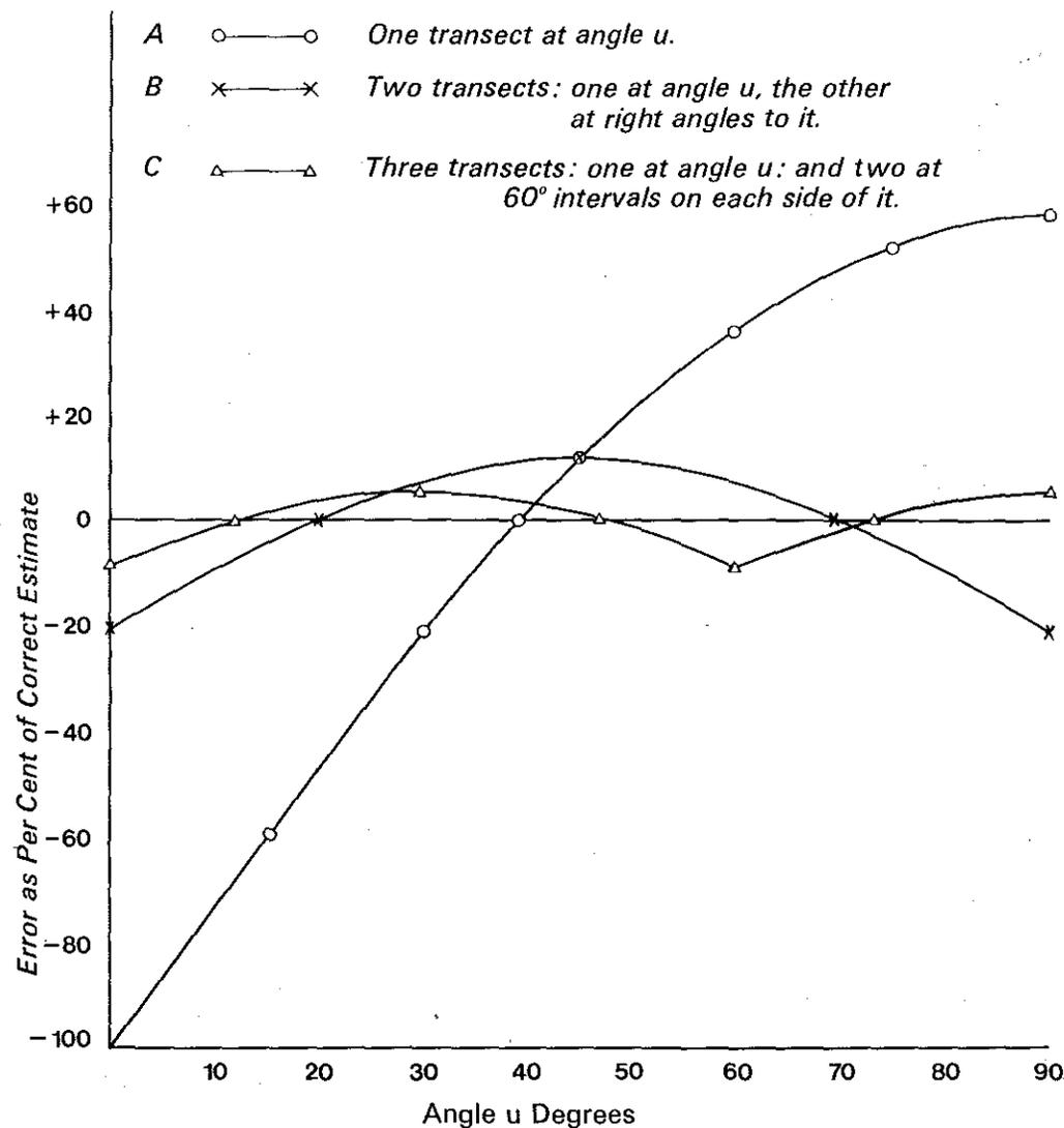
FIGURE 2. Extreme possible errors in the line intersect method for one, two and three sample lines at uniform angular intervals.
